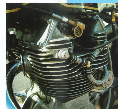
Rev counter drive is taken from the left hand side of the engine.
