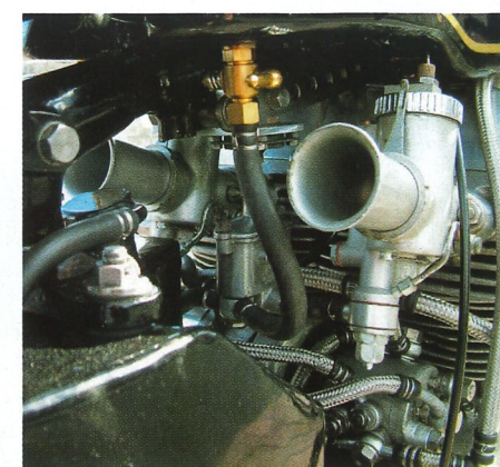
Twin carburetors are by Amal, though due to availability not as fitted in the machine's racing days.
